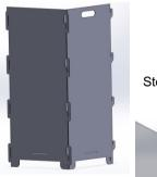
Step 1: Fit sides 1 and 2 together using slot-in connection system.
